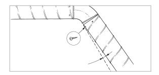
Mount the next piece of duct at an angle, but make sure that the rubber sealant is not visible. Put screws or blind rivets where the notches have not clicked in position.
