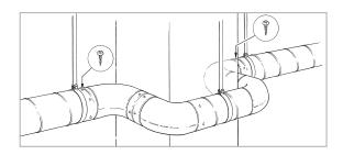
In situations where the mounting must be locked, e.g. when a bend is mounted to a duct and it twists downwards the floor. Mount the first hanger and mount the bend, then lock the joint with a screw or blind rivet.
