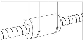
Depending on size and weight the suspension of the circular ducts/silencer should be strengthened by means of hangers to prevent it from falling down. Mount the hangers in a straight line and as close to every joint as possible. Fix with an extra screw when needed for extra stability.
